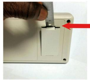
Gently pry the battery compartment lid open with a flat tool to access the battery for replacement.
